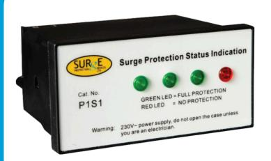
This surge protection status indication module is easy to install with any of our surge protection devices that are designed with a volt free change over contact.
